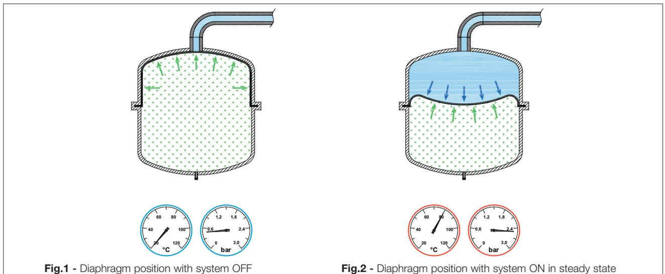
**Fig.1** - Diaphragm position with system OFF
